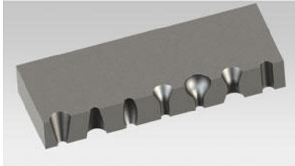
Figure 3: The types of hole cross-sections that are feasible to manufacture using laser drilling.
